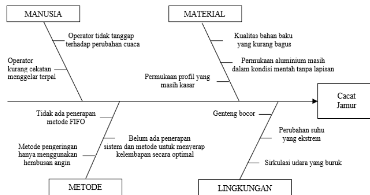
Figure 7. Fishbone Diagram for Mold Defect
